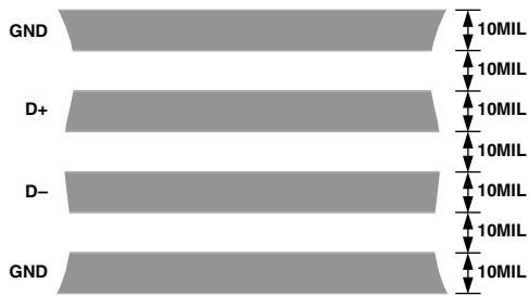
Figure 8. Arrangement of Signal Tracks
